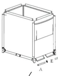
These sleeves can open to easily install the tubes.
