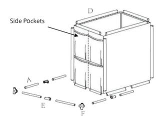
Attach the tubes from step 1 to the 3-way side connectors (E) from step 2.
