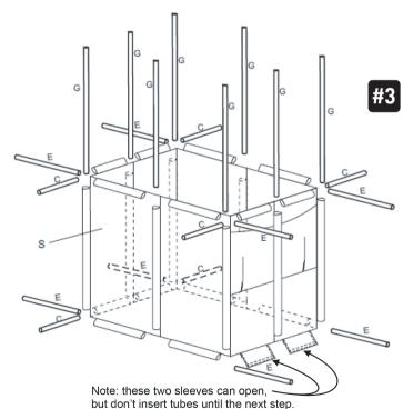
Insert six Tubes (C), eight Tubes (G), and eight Tubes (E) in the Lower Mesh Bag (S).
