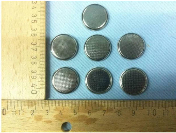
Cell/电芯 (CR2025 3,0V 150mAh)
